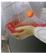
To fill the CellSTACK vessel by hand, tilt the vessel slightly toward the filling port. Smaller CellSTACK vessels can also be emptied by hand by carefully pouring from the filling port into a sterile collection vessel.
