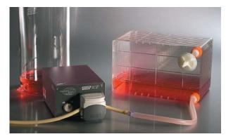
If using a peristaltic pump for filling and emptying, it is recommended to replace the vent cap with a venting filter to prevent potential shearing, media foaming, or cracking of the vessel.
