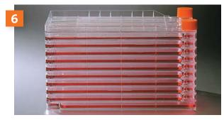
For additional gas exchange during incubation, one or both venting caps can be replaced with a higher gas flow filter. Place the CellSTACK vessel into an incubator or warm room.
