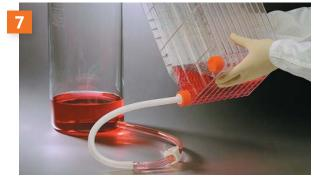
To empty the CellSTACK vessel, replace one of the vented caps with a filling cap as in Step 2. Ensure the CellSTACK vessel is above the sterile collection vessel if emptying by gravity.
