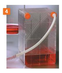
Once filling is complete, turn the CellSTACK chamber 90° so that the filling and venting ports are up (as shown). It is normal for the medium level in the bottom chamber section to be slightly higher. Replace the filling cap with the original vented cap and the vented cap with a venting filter or solid cap (Cat. No. 3969).
